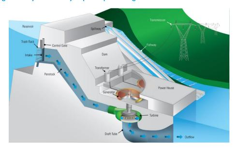
Figure 7. Key factors in hydropower plant design
