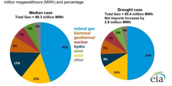
Figure 9. Forecast June–September 2022 California generation mix, Median case versus Drought case
