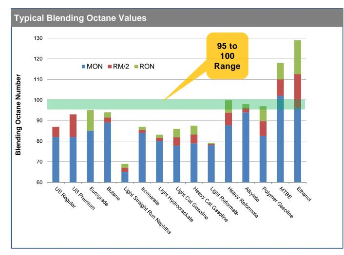
Very few refinery components exceed 95 RON – limiting the capability of refiners to improve pool octane to that level
