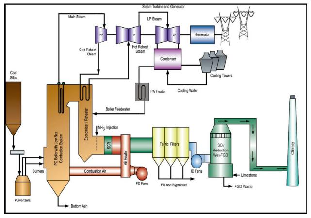
FIGURE 4-1 – USC FACILITY DIAGRAM
