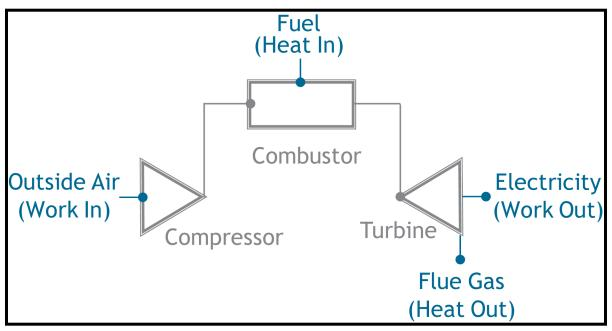
FIGURE 10-1 – CONVENTIONAL CT DESIGN CONFIGURATION
