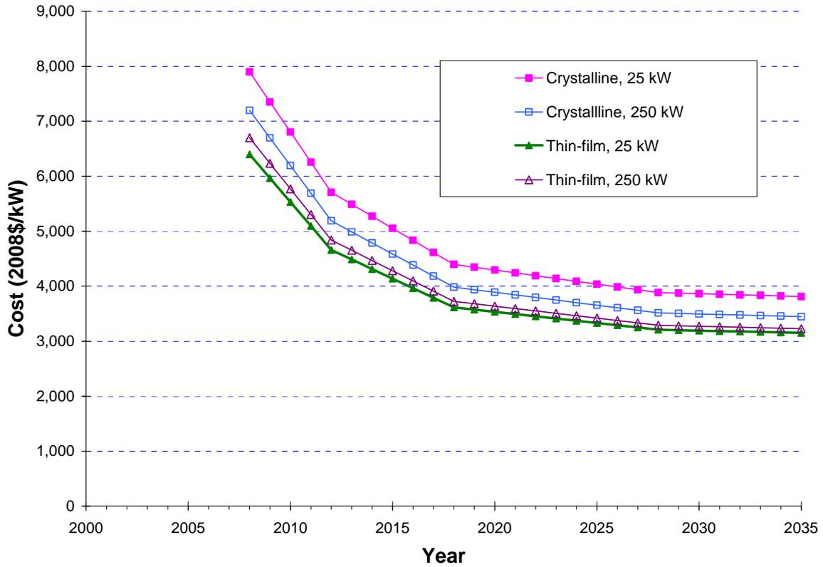
**Figure 20. Commercial Installed Capital Costs, Reference Case**
