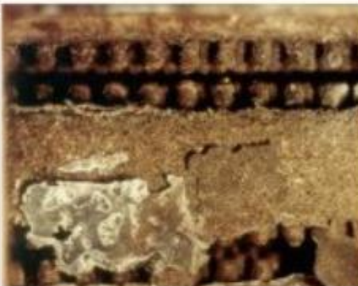
No. 2 heating fuel, 1.08% sulfur
