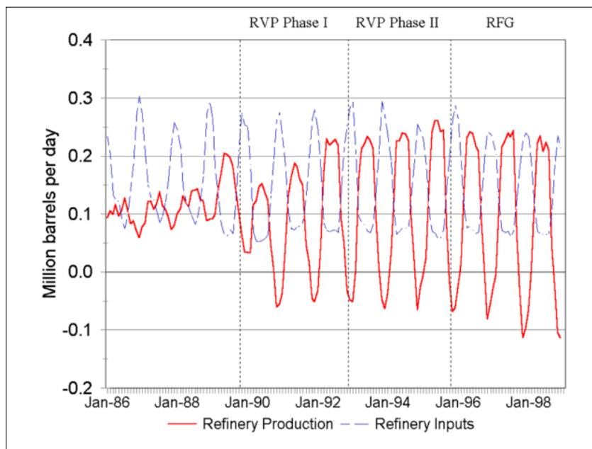
It is not surprising that the observed reduction in net refinery inputs of LPGs during the summer RVP control periods are lower than what is implied by the simple linear vapor pressure blend calculation noted above. First, not all gasoline supply was affected by each regulation. Second,
