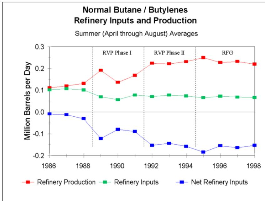
The dramatic change in refinery operations is very evident in a graph of refinery inputs and production of normal butane ([Figure 1](#)).
