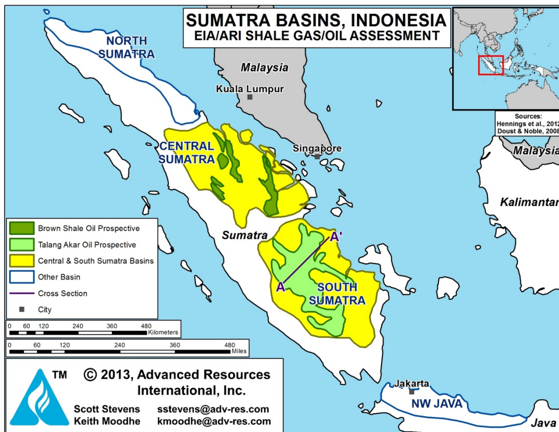
Figure XXIII-3. Prospective Shale Areas in the Central and South Sumatra Basins, Indonesia.
