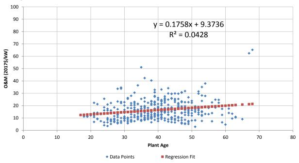
Figure B-8 — Gas/Oil Steam Dataset – O&M for Greater than 1,000-MW Plant Size
