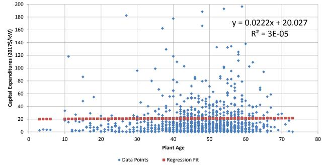
Figure A-11 — Coal Steam Dataset – CAPEX for All Plants with Avg. Net Capacity Factor < 50%
