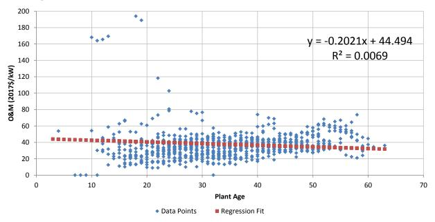
Figure A-8 — Coal Steam Dataset – O&M for 1,000-MW to 2,000-MW Plant Size
