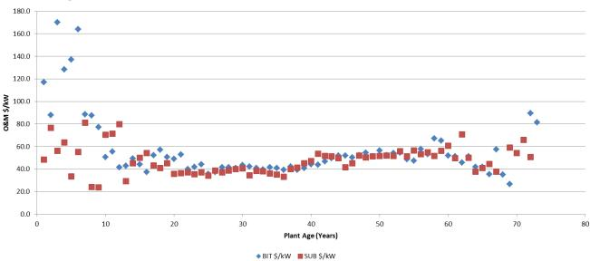
Figure A-20 — Coal Steam Dataset – O&M for Bituminous vs. Subbituminous
