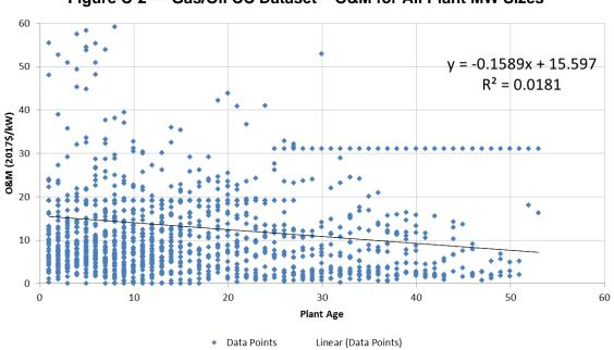
Figure C-2 — Gas/Oil CC Dataset – O&M for All Plant MW Sizes
