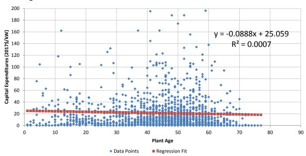
Figure A-3 — Coal Steam Dataset – CAPEX for Less than 500-MW Plant Size
