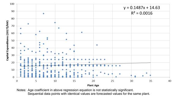
Figure C-11 — CC Dataset – CAPEX for All Plant Sizes and Avg. Net Capacity Factor > 50%
