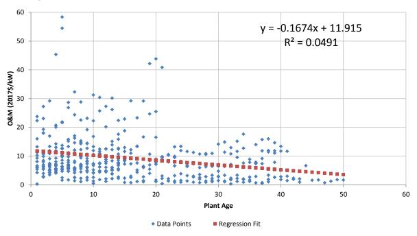
Figure C-6 — Gas/Oil CC Dataset – O&M for 500-MW to 1,000-MW Plant Size
