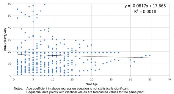
Figure C-12 — CC Dataset – O&M for All Plant Sizes and Avg. Net Capacity Factor > 50%
