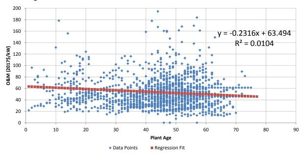
Figure A-4 — Coal Steam Dataset – O&M for Less than 500-MW Plant Size
