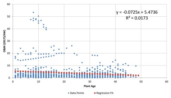
Figure D-8 — Gas/Oil CT Dataset – O&M for Greater than 300-MW Plant Size
