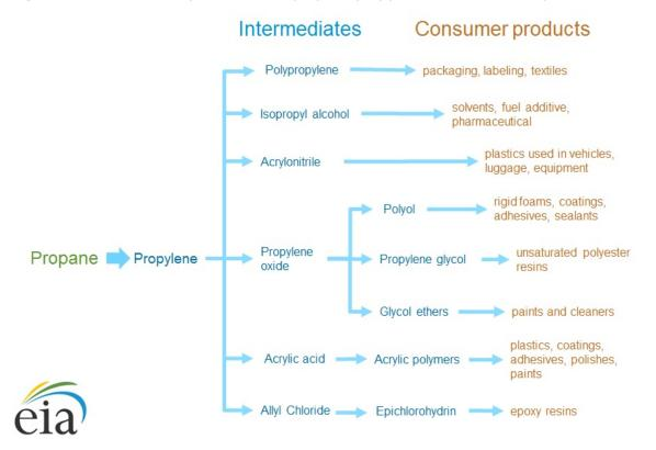
Figure 16. Petrochemicals produced from propane/propylene as feedstock (simplified)
